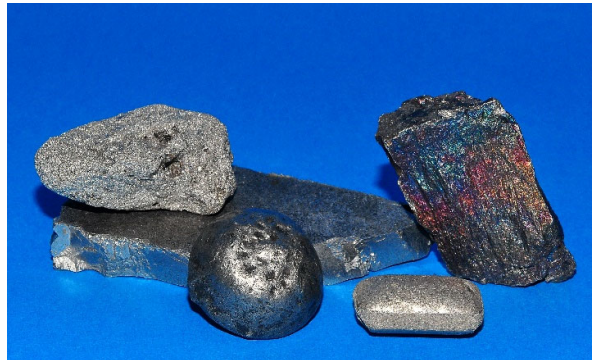
Fig. 2 How elements are added to the molten steel: As pure metals (oxidation level 0 = zero), or as pre-alloys, such as Cr-Fe, Ni-Fe, Mo-Fe etc. In such pre-alloys, the metals are always in oxidation level 0. To the left are two Cr-Fe alloys (50-80 % Cr), the Ni-Fe (50 % Ni), anode nickel (99 % Ni), and Mn-Fe (> 50 % Mn).
